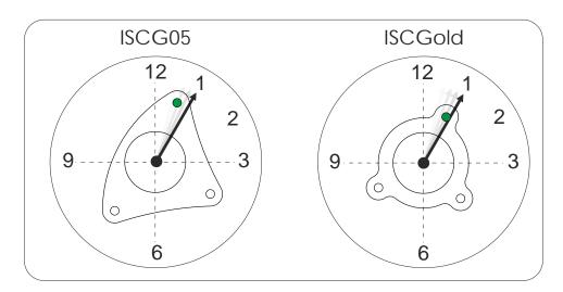
**4.** Tighten the bottom bracket cups using wrench, while making sure that the adaptor has not changed its position.
